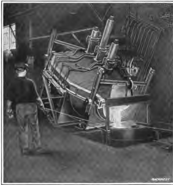
Fig. 8. Ten-ton Ludlum Furnace in Pouring Position
